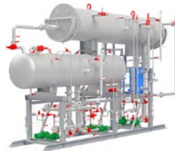
Fig. 2: STEP model of a Flux-Hi™ cascade system, Holger Andreasen & Partner GmbH
