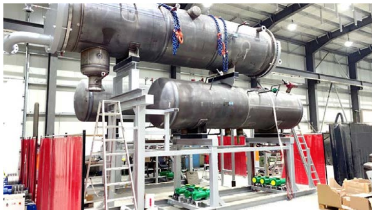
Fig. 1: Layout of the Flux-Hi™ \text{NH}_3 / \text{CO}_2 cascade installation in Berlin 2020, Holger Andreasen & Partner GmbH
